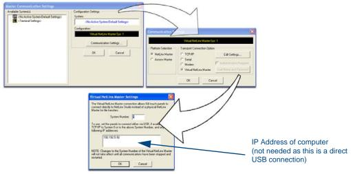
FIG. 28 Assigning Communication Settings for a Virtual Master
